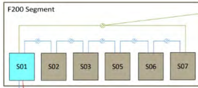
Figure 301-6: TPSS Transfer Trip Network Ring Topology Example
