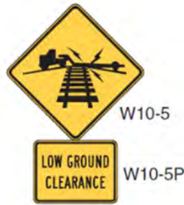
Figure 120-18: LOW GROUND CLEARANCE Sign
