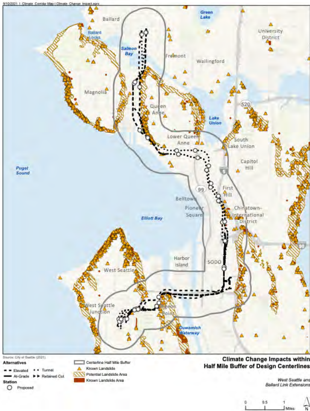
Figure 4-9. Map of Known Landslide Locations and Potential Landslide Areas within Half Mile Buffer of Proposed WSBLE Alternatives
