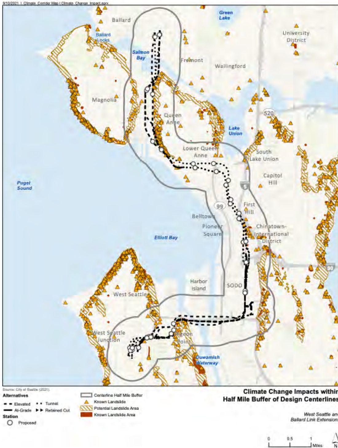
Figure 4-5. Map of Known Landslide Locations and Potential Landslide Areas within Half Mile Buffer of Proposed WSBLE Alternatives
