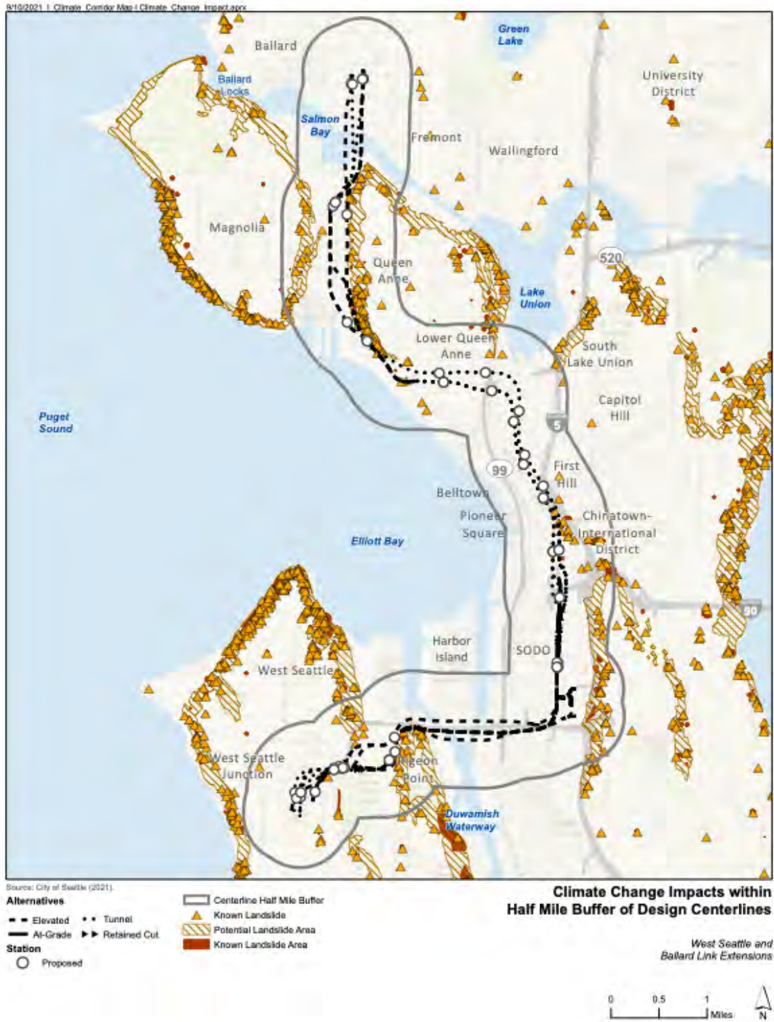
Figure 2-1. Map of Known Landslide Locations and Potential Landslide Areas within Half Mile Buffer of Proposed WSBLE Alternatives
