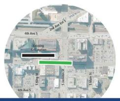
Station location alternative (straddle S Jackson St) Note: applicable to both cut and cover and bored tunnel alternatives
