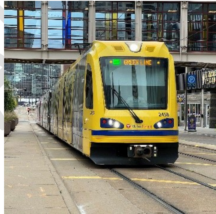
Figure E-11 Wig Wag Train headlights as implemented by Metro Transit
