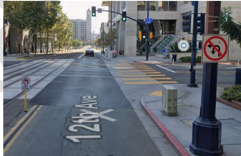
Figure E-15 Example of eye-level “NO LEFT TURN” signage and delineator
