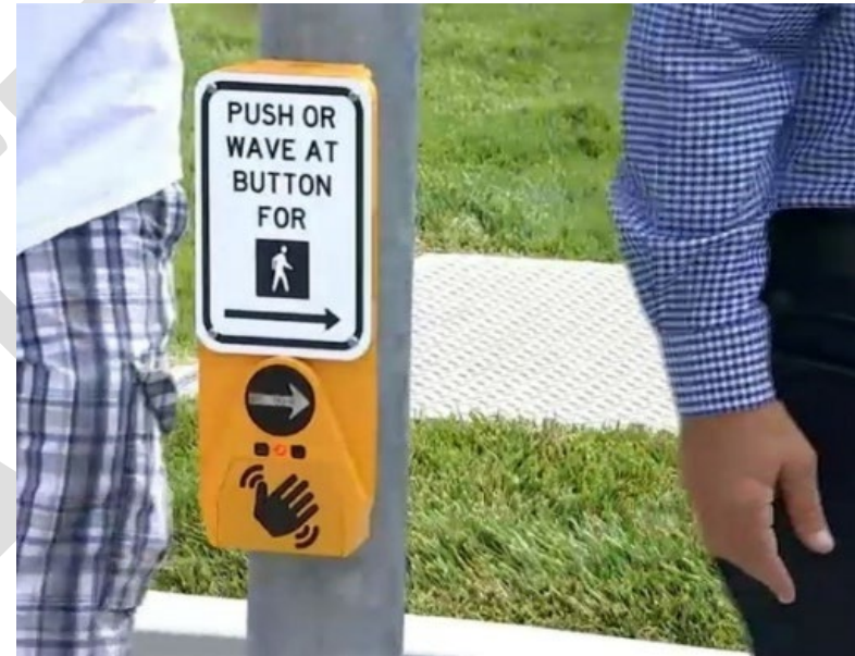
Figure E-14 Touchless pedestrian push button
