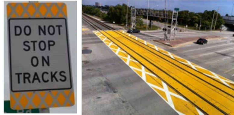
Figure E-2 (left) Sample DO NOT STOP ON TRACKS signage Figure E-3 (right) Sample dynamic envelope pavement markings
