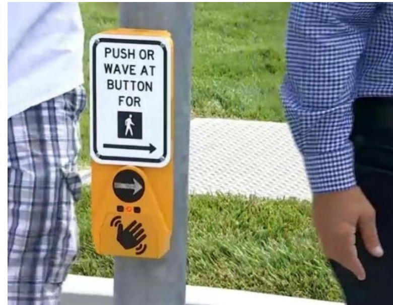
Figure E-5 Touchless pedestrian push button
