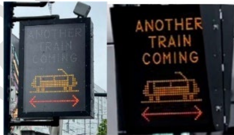
Figure E-16 ATC Current Blank-Out Sign
